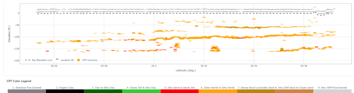
Figure 8. CPT stratigraphy profile with user-defined rules to identify and visualize critical soil design layers [71]
