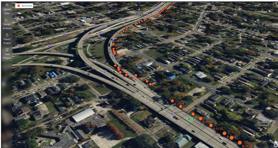
Figure 14. 3-D interactive map view displaying deep soil boring locations imported from a gINT file onto the web-based platform
