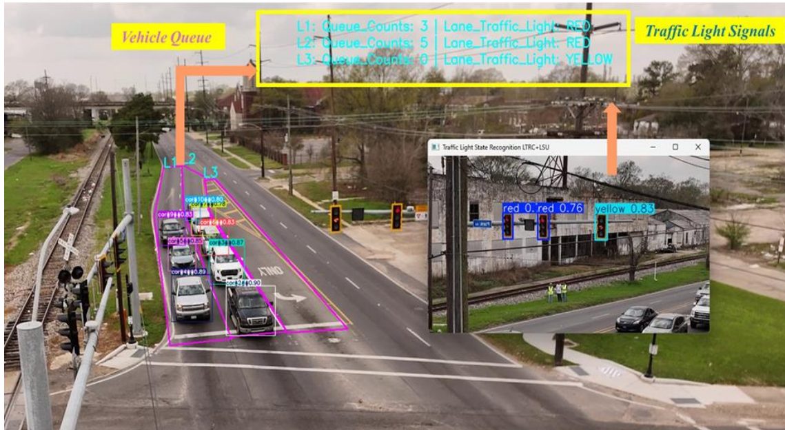
Figure 38. Visualization of queue length estimates and traffic light states at Plank Road at Choctaw Drive
