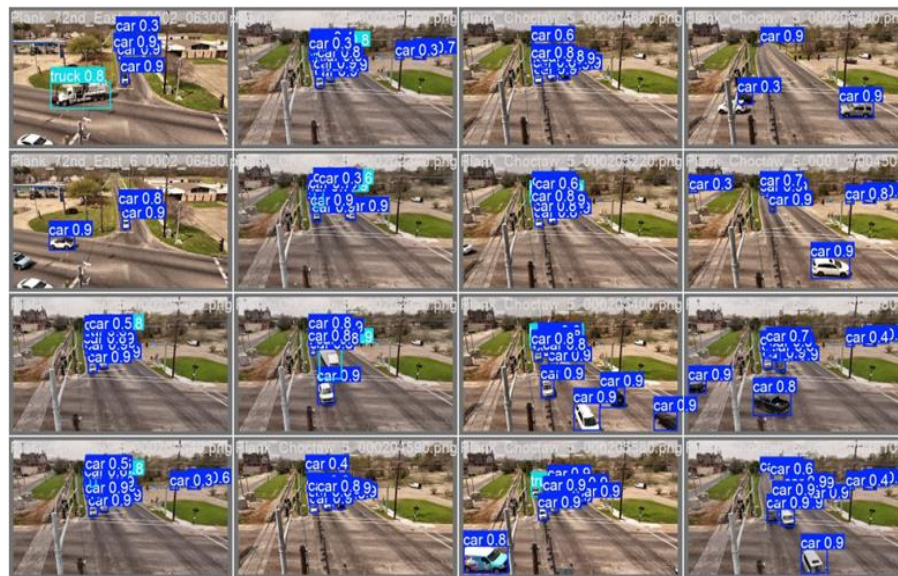
Figure 2. Sample test of the vehicle detection model
