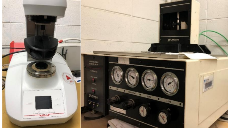
Figure 4. Anton Paar MCR 72 with mechanical gear system and Bending Beam Rheometer
